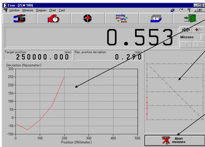
The diagram shows the readings so far taken on a measuring line.
