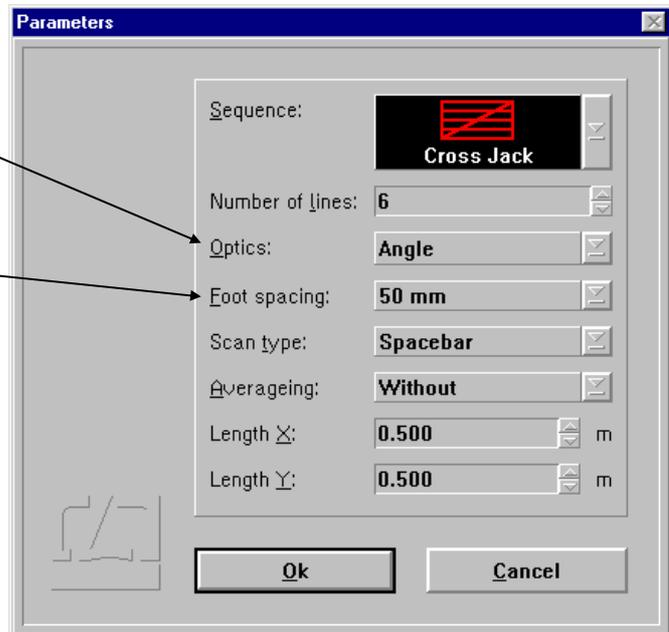
In the "Scan type" list box you can select the event to trigger data acquisition, i.e. either by hitting the space bar of the computer keyboard or by an external signal (remote control).
