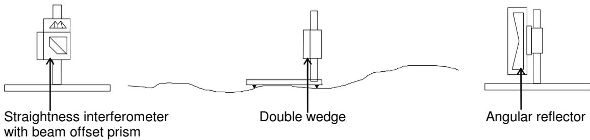
The program directly measures the displacement of the double wedge normal to the plane.
