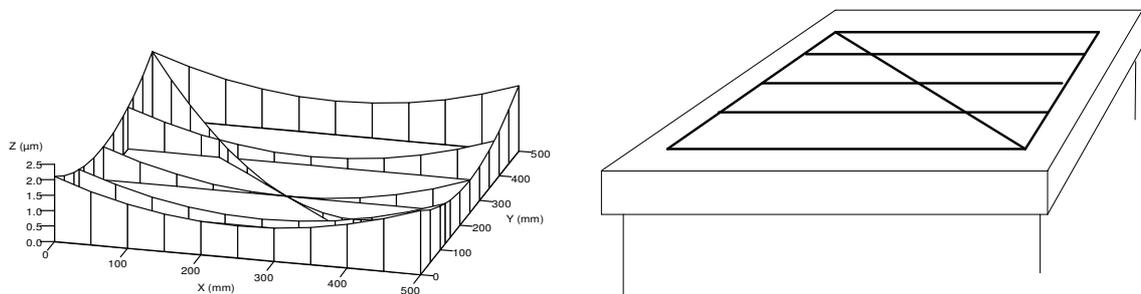
To determine the deviations normal to the plane, you can use either the angle or straightness optics, same as in straightness measurement. Use of the angle optics involves less mounting work. Mount the double reflector on a base distance plate. During a measurement, displace the base distance plate repeatedly along a measuring line by the distance between the two rest points of the plate.
