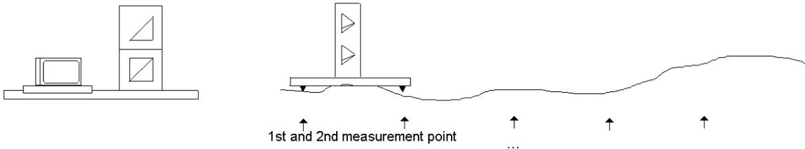
Straightness optics: The double wedge is above the first measuring point.
