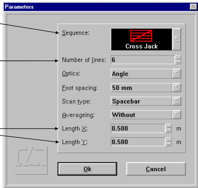
In the **"Optics"** drop-down list box you can select between using angle optics and the 2m or 10m straightness optics. If you use angle optics, you need to specify the base distance plate to be used. The value set here determines the interval of the grid of measuring points, no matter whether you use angle or straightness optics.
