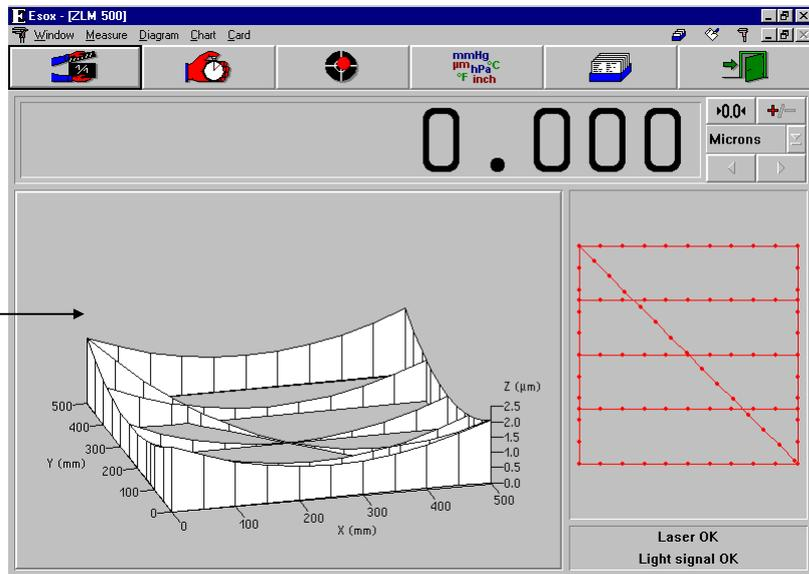
Tilt, rotation and height (Z expansion) of the diagram shown can be changed in the text input boxes in the top left portion of the window.
