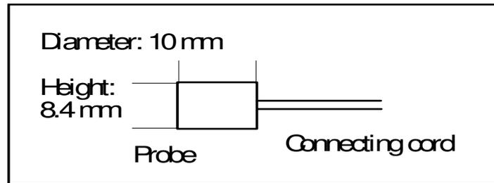
The sensors are delivered in series with cable lengths of 5 m. Other lengths will be supplied on request. The sensors are hermetically sealed and will therefore withstand rough conditions in production environments.
