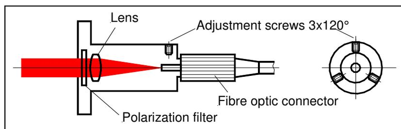
Fig. 42: Fibre optic coupling with adjustment screws
