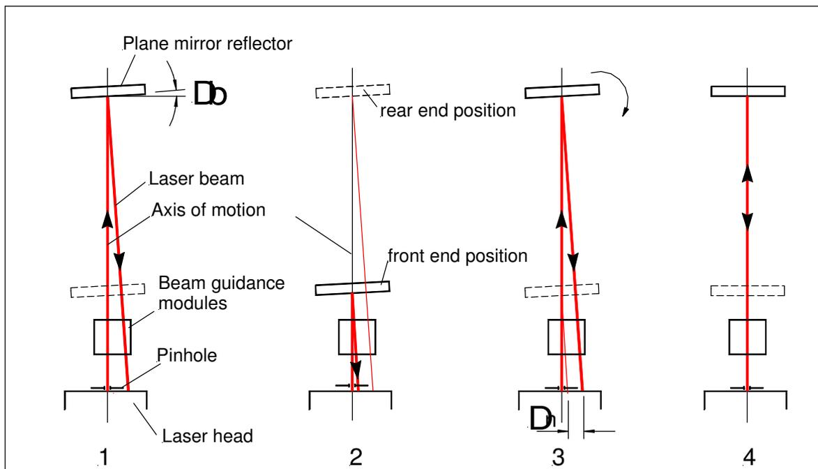
Fig. 40: Adjustment of the plane mirror reflector to the motion axis
