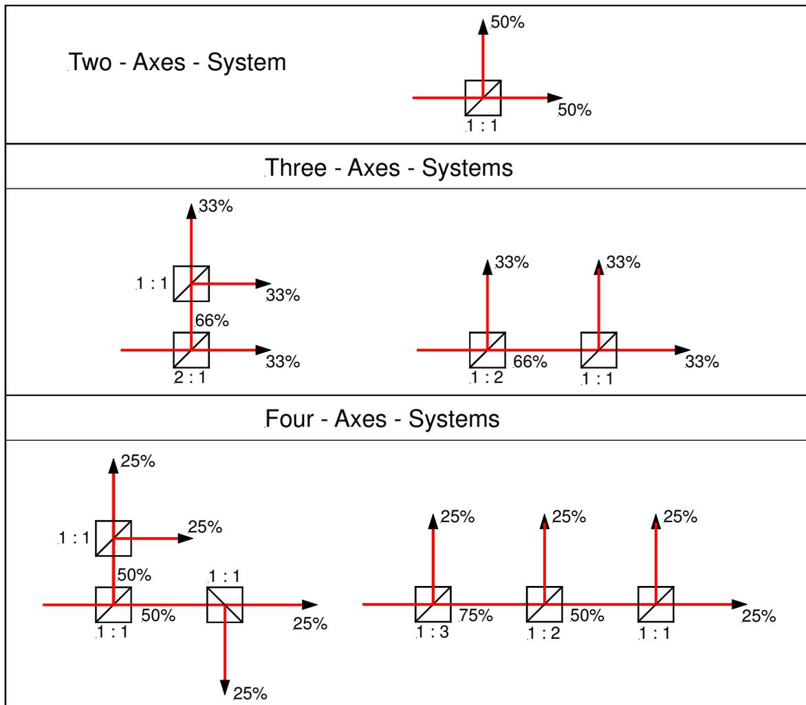
Fig. 27: Example of possible variants of beam splitting in multi-axis systems
