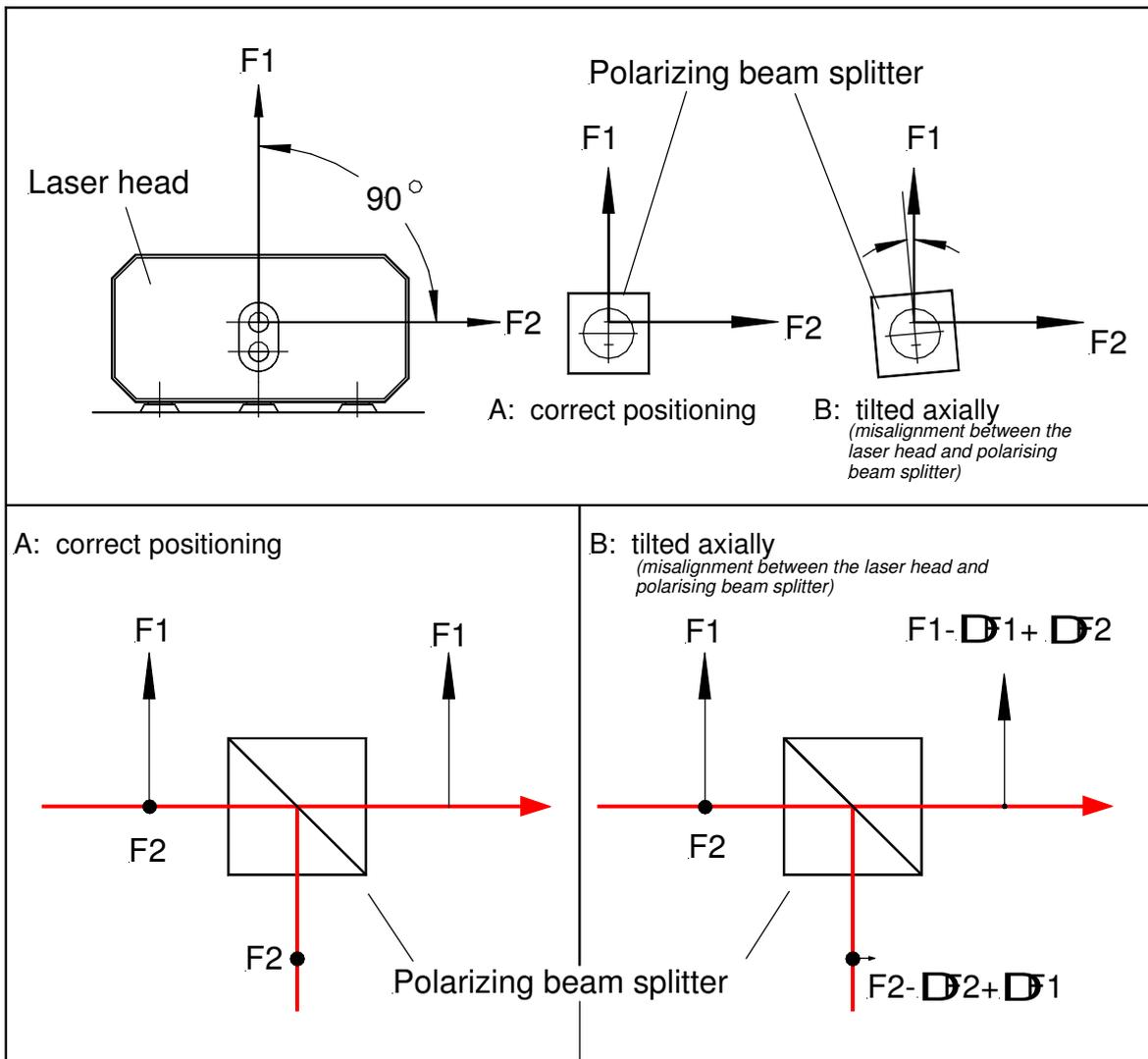
Fig. 30: Mixing of modes by rotation of the interferometer to "polarization cross "
