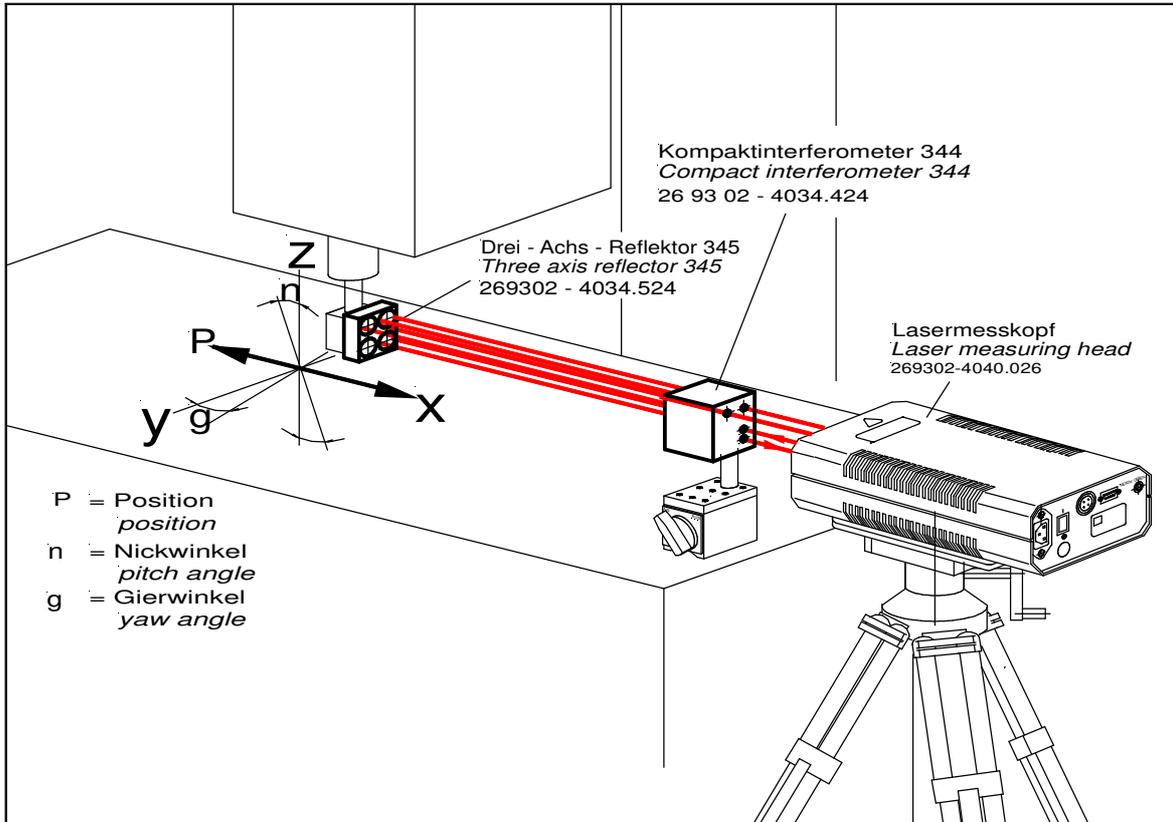
Fig. 22: Simultaneous position, pitch angle and yaw angle measurements in one axis direction
