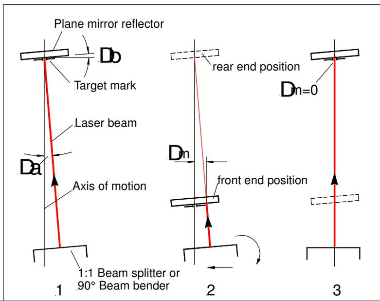
Fig. 39: Adjusting the beam direction of the laser beam to the movement direction of the axes of the XY-stage
