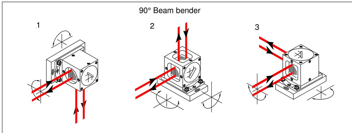
Fig. 31: Installation and adjustment possibilities of modules size A (□ 40) for beam guidance
