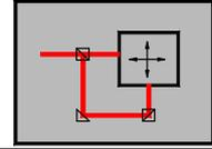
Fig. 22 shows a measurement assembly of a machine. For the correction of the comparator error are measured position, pitch angle and yaw angle in one axis direction simultaneous.
