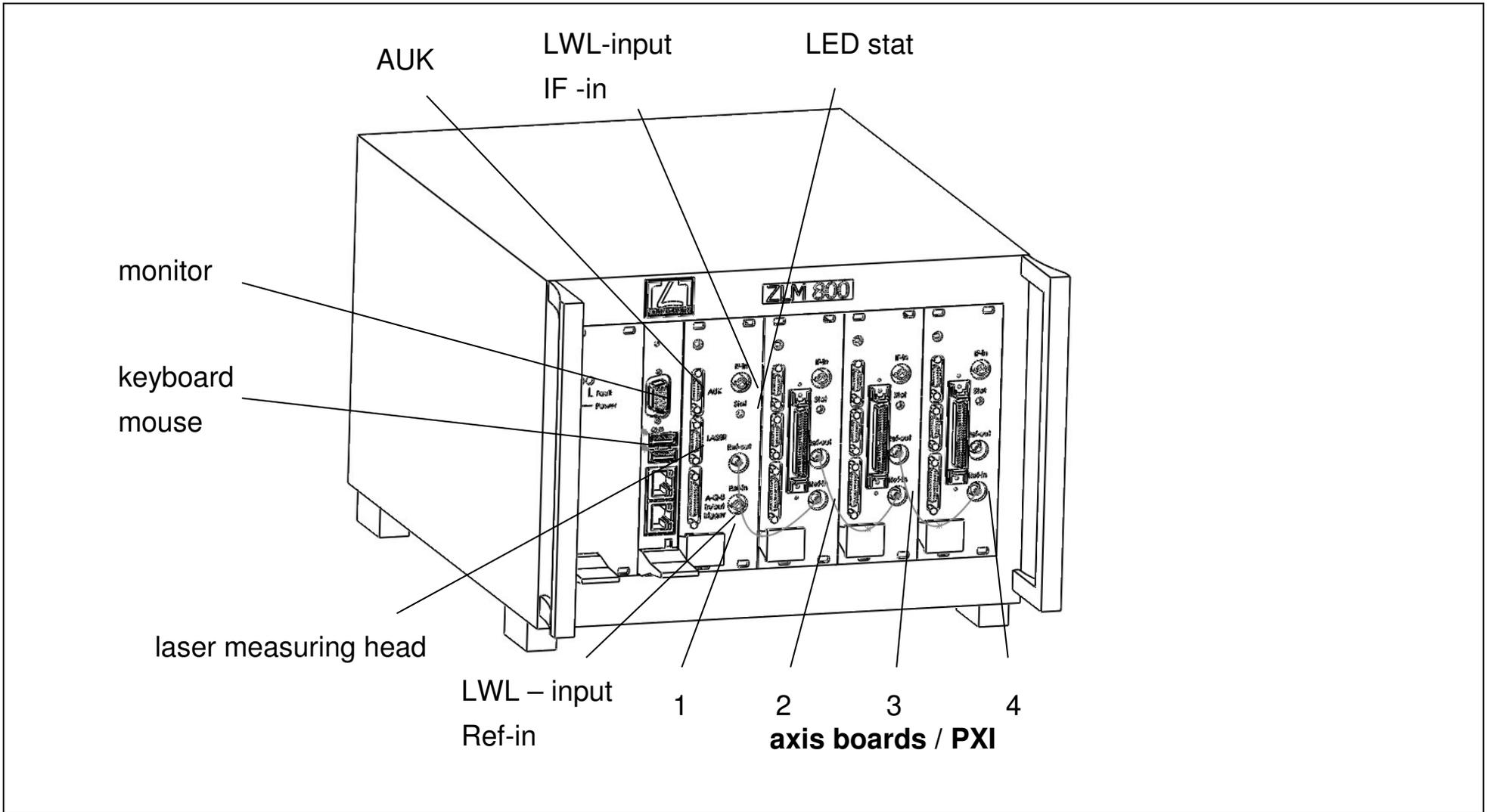
Fig. 26: Evaluation unit ZLM800 cPCI/PXI
