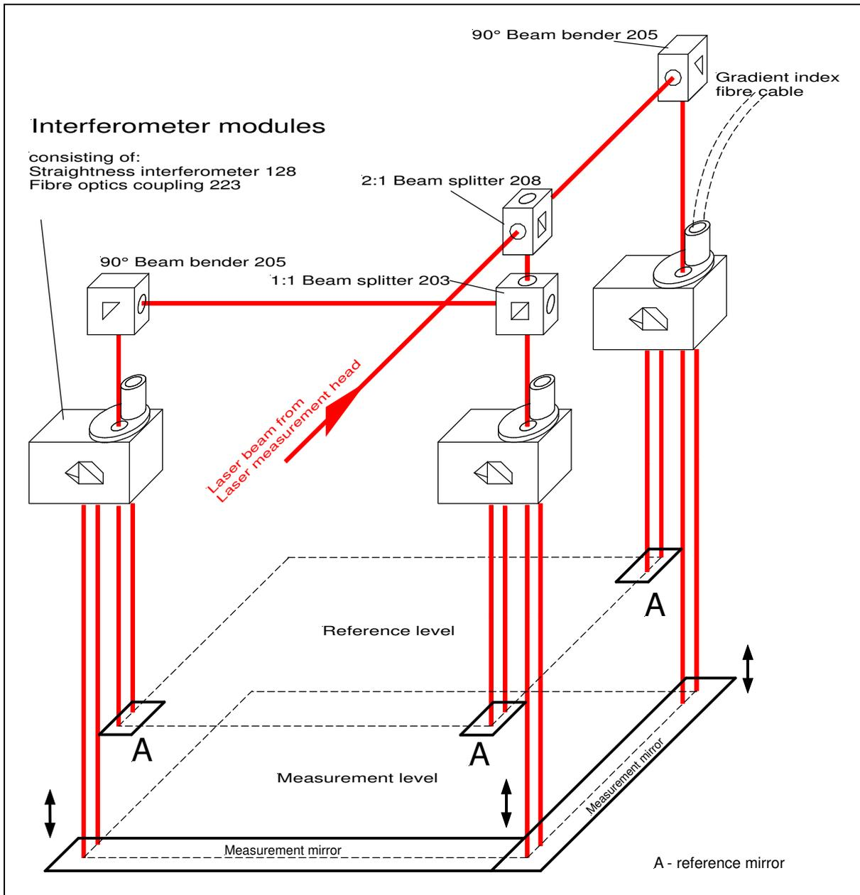
Fig. 12b: Multi-axis-arrangement (3 axes) realised with Differential interferometer 128
