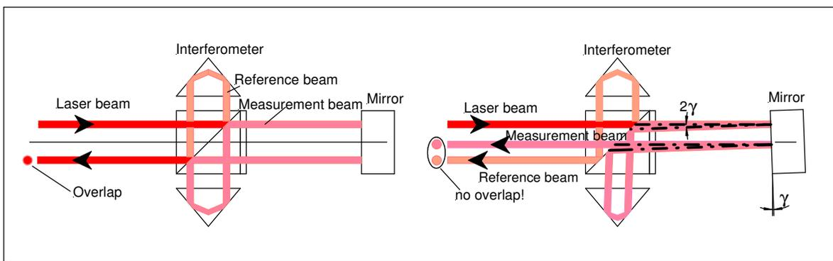
Fig. 28: Overlap of measurement and reference beam
