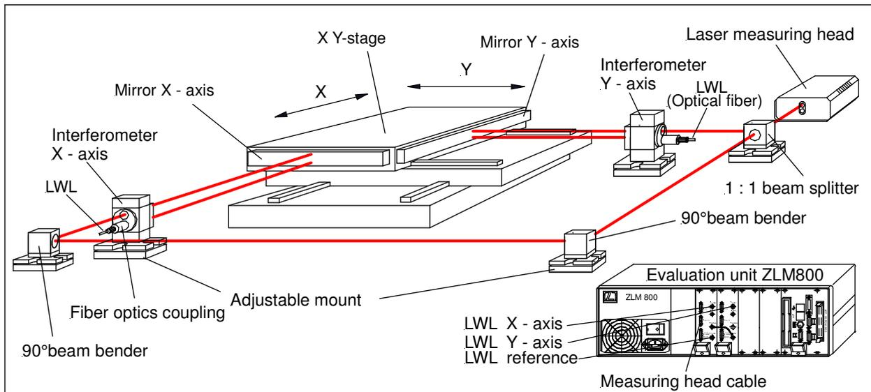
Fig. 1 : Configuration of a two-axis systems with plane mirror interferometers
