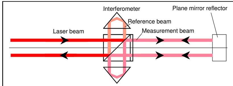
Fig. 41: Plane mirror interferometer
