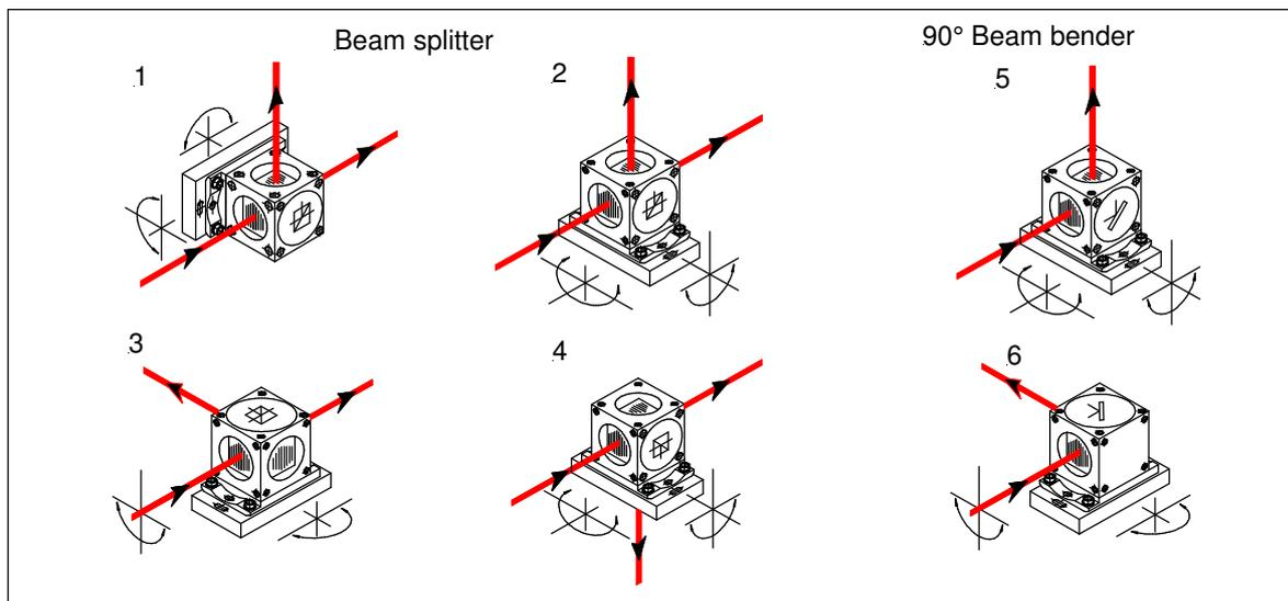
Fig. 32: Installation and adjustment possibilities of modules size B (□28, □20 ) for beam guidance
