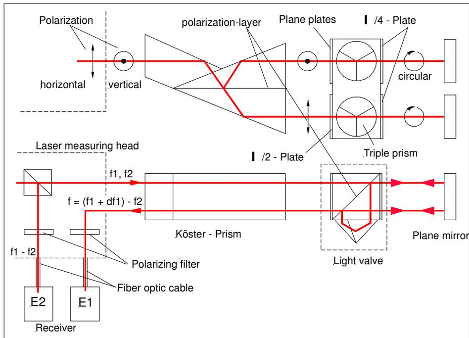
Fig. 18: Functional principle of parallel interferometer ("Köster interferometer")
