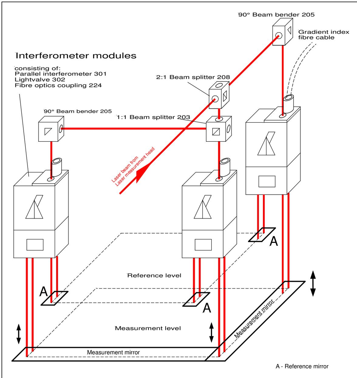
Fig. 12c: Multi-axis-arrangement (3 axes) realised with Parallel interferometer 301
