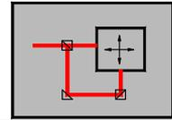
First, the laser head and the beam-guiding optics modules, 1:1 Beam splitter and 90 °Beam bender, are mounted (see fig. 37a).
