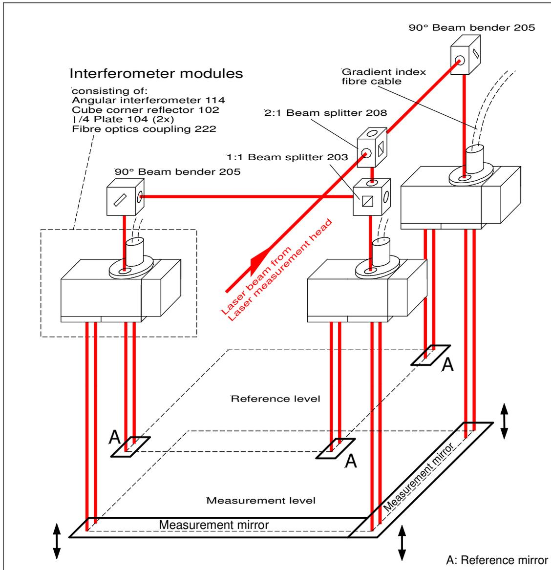
Fig. 12a: Multi-axis-arrangement (3 axes) realised with Angular interferometer
