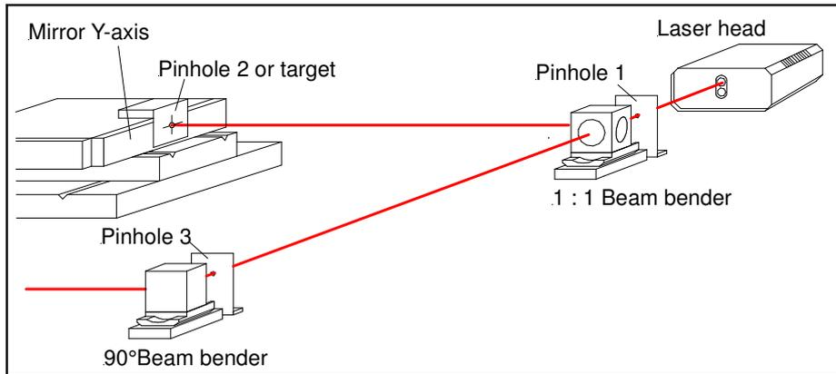
Fig. 38 Alignment of the beam heights by using pinholes
