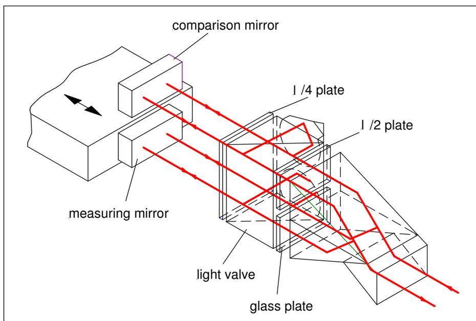
Fig. 17: Schematic diagram of the interferometer optics for difference plane mirror interferometers
